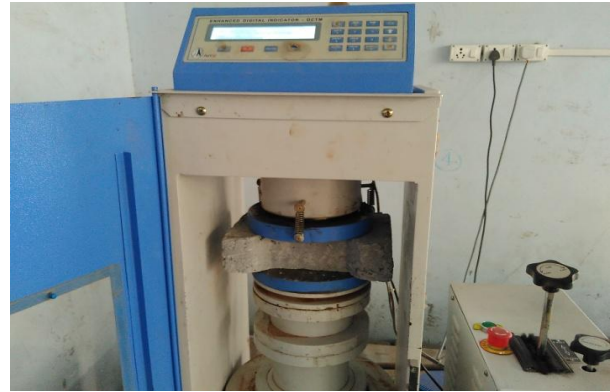
Fig. 2. Compressive strength on paver blocks
