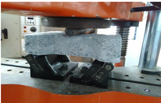
Fig. 4. Flexure strength on paver blocks
