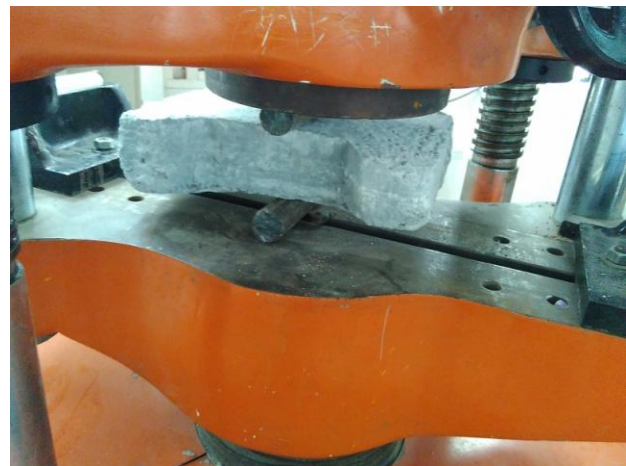
Fig. 3. Split tensile strength on paver blocks
