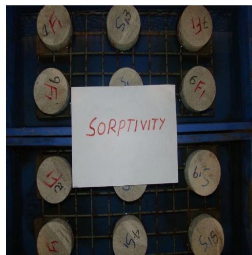
Fig 9 cubes under sorptivity test
