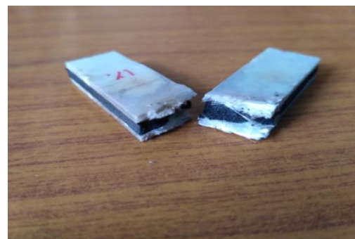
Fig.4. Izod impact tested sample (1 wt. % of TiO 2 )
