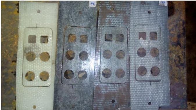
Fig.2 Finished and cut samples having (a) 0, (b) 1, (c) 2 and (d) 3 wt% of Silicon carbide.
