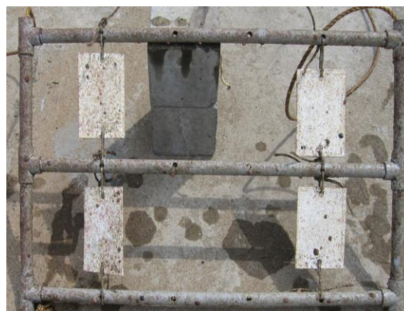
Fig. 4. Image of panels exposed in sea water for 3months.
