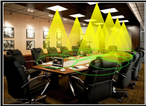
Fig. 2: Multiple Li-Fi APs in a room
