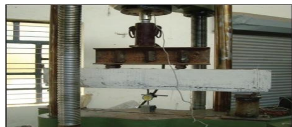
Figure 2 Flexural strength test setup for beam
