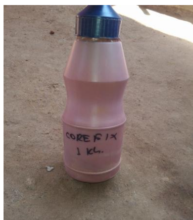
Fig 9: Core fix (Para-Toluene Sulphonic acid)
