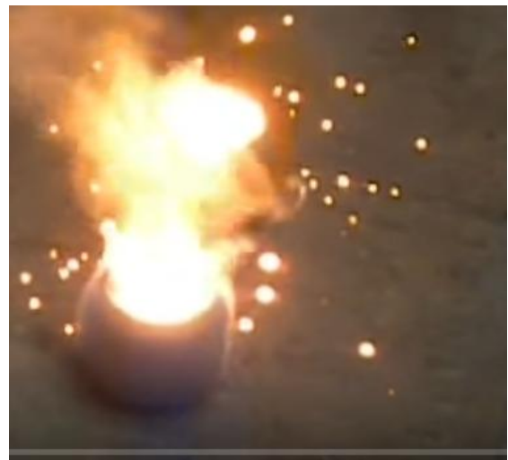
Fig 13: Exothermic sleeve during testing
