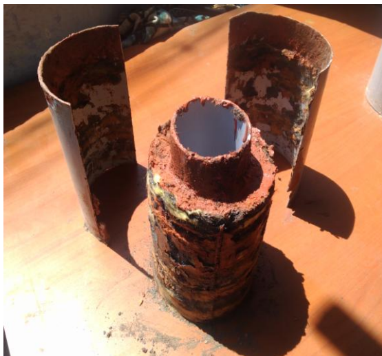
Fig 12: Finished exothermic sleeve
