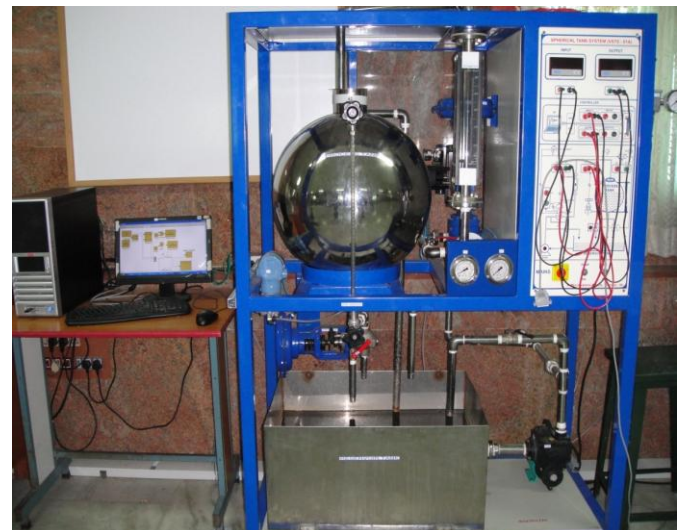
Fig 2 Spherical tank setup
